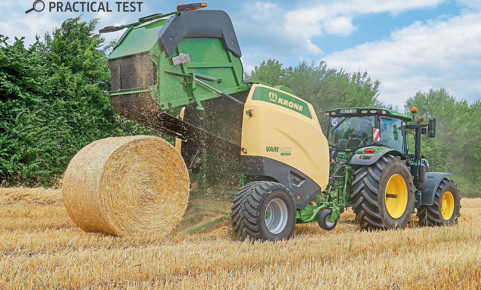
Straw was the main crop we tackled with the VariPack V190XC Plus variable-chamber belt baler in our practical test.
