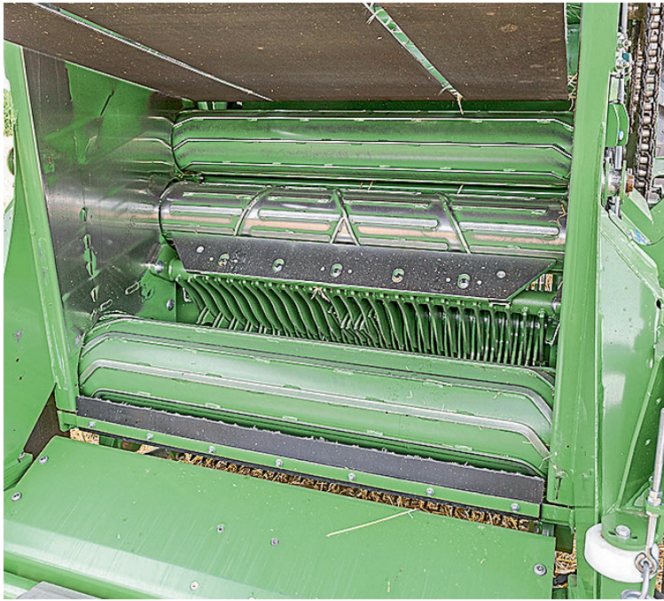
Three rollers and three belts ensure material is compressed right from the off.
