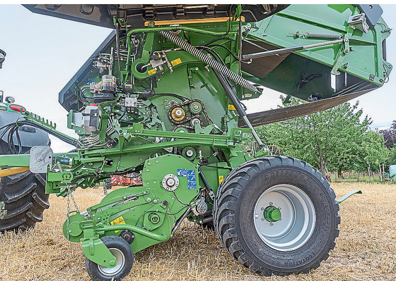
The automatic oiler and lubrication systems are located on the left-hand side of the machine. On the right-hand side is the drive for the rotor and pick-up.
