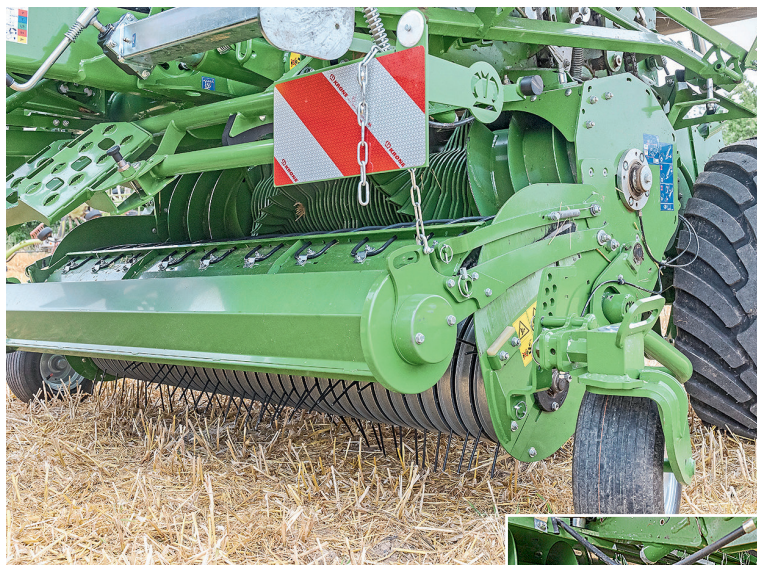
The tines on the pick-up are arranged in a helical pattern, and there's an effective crop roller, too. The rotor has integrated augers on the sides.
