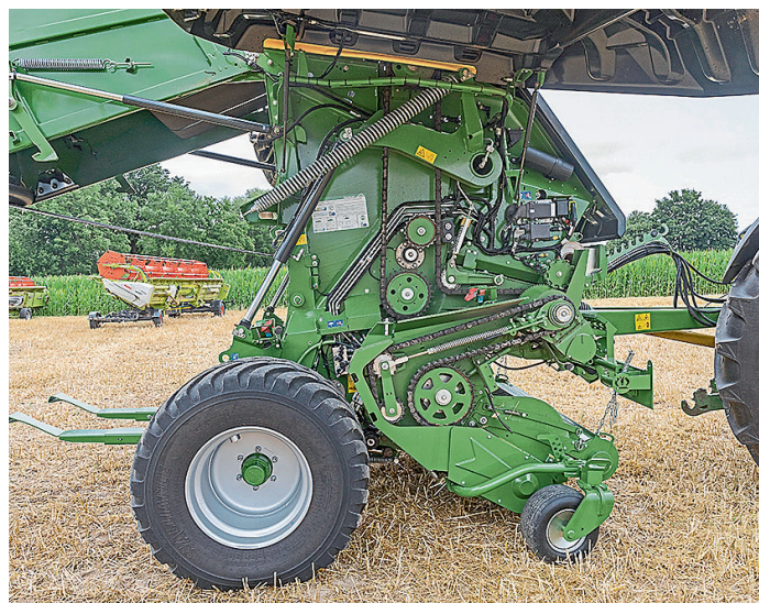
The automatic oiler and lubrication systems are located on the left-hand side of the machine. On the right-hand side is the drive for the rotor and pick-up.
