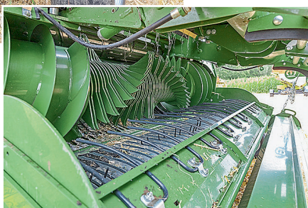
The tines on the pick-up are arranged in a helical pattern, and there's an effective crop roller, too. The rotor has integrated augers on the sides.
