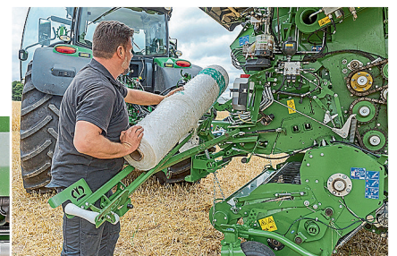
Threading the net is relatively straightforward, and the pivoting side chute makes loading a fresh roll a lot easier.
